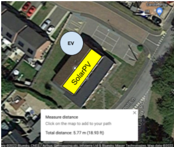
Proposed 18kWp SolarPV array on Hall
