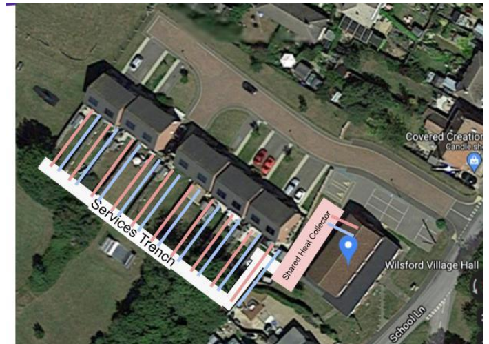
The shared ground collector scheme
