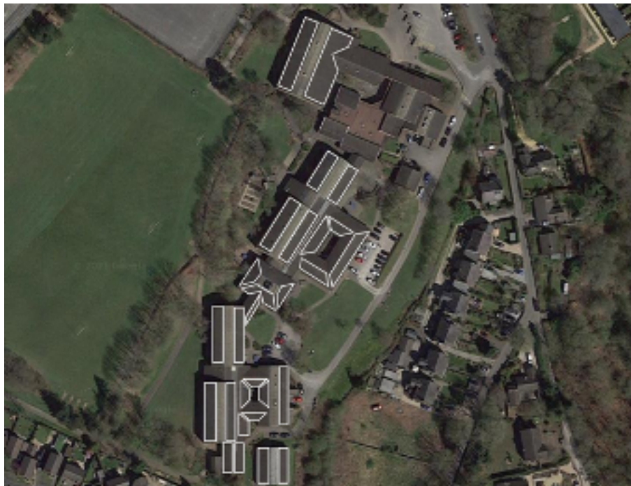
FIGURE 4- AERIAL VIEW OF HIGHFIELDS UPPER SITE; SUITABLE ROOFING AREA OUTLINED IN WHITE
