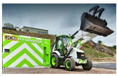
JCB Hydrogen ICE prototype loader
