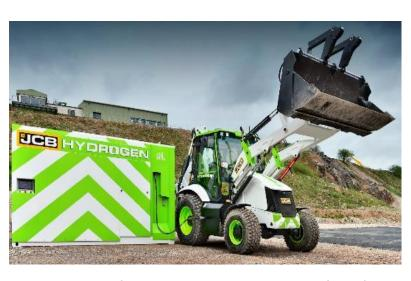
JCB Hydrogen ICE prototype loader
