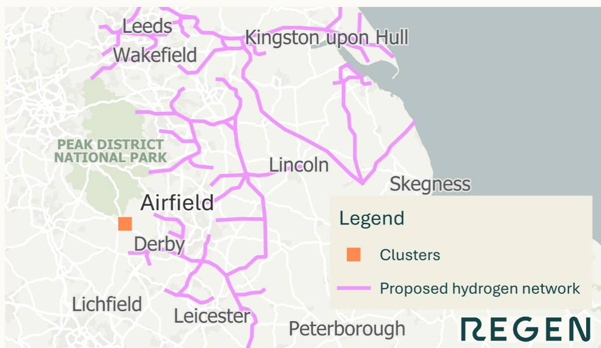
Figure 17: Map showing the Airfield cluster against the proposed hydrogen transmission network from the East Coast Hydrogen project. East Coast Hydrogen – Pipeline North Phase 1 NZASP Re-opener , Cadent Gas, 2024; Map data from OpenStreetMap .
