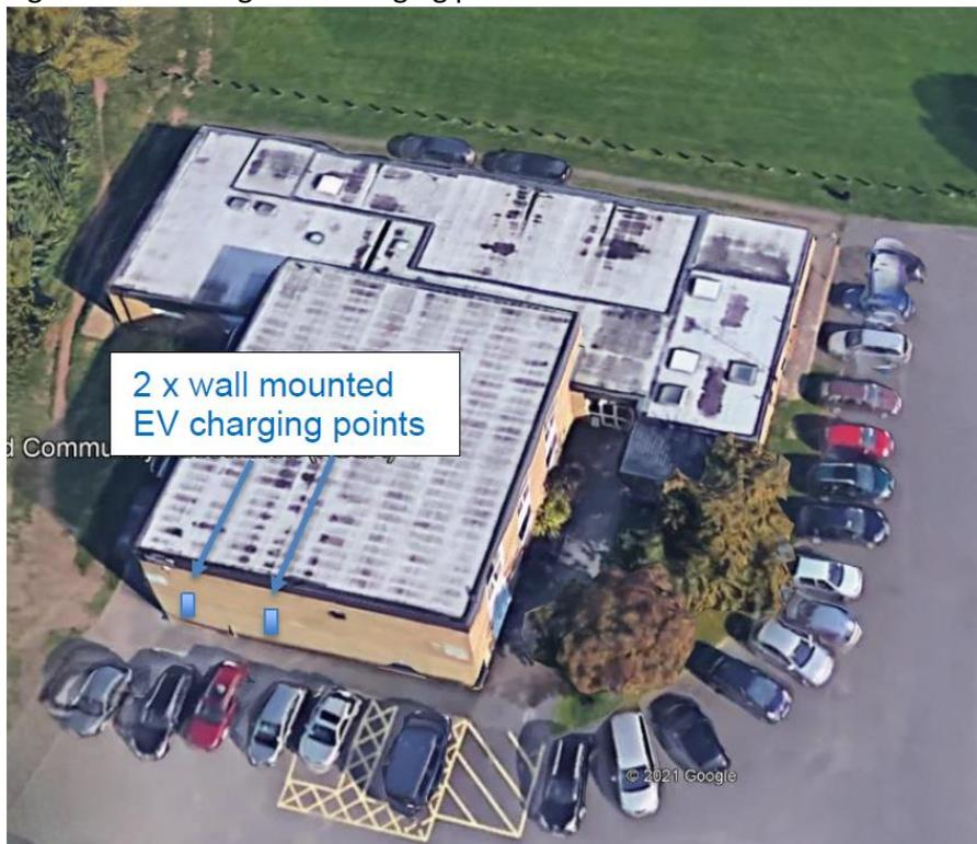
The above photograph illustrates proposed position of 2 EV charging points in an easily accessible area of the car parking and near the disabled spaces. It is readily accessible to electrical services
