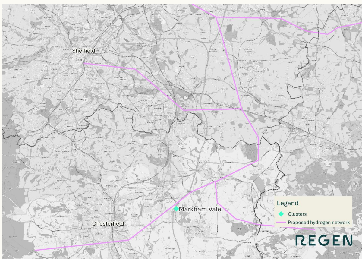
Figure 29: Map showing Markham Vale against the proposed hydrogen transmission network from the East Coast Hydrogen project. East Coast Hydrogen – Pipeline North Phase 1 NZASP Re-opener , Cadent Gas, 2024; Map data from OpenStreetMap .
